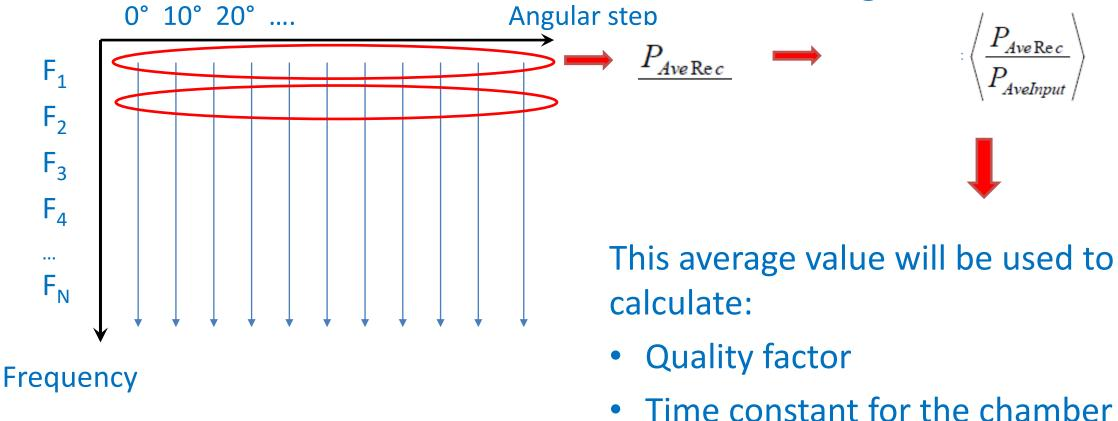
The power to generate for the test (depending on standard) <sup>16</sup> 4.1 Measurement of Power received in the chamber
